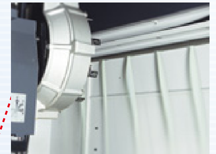
Chip shower Chip shower located at the upper section inside the machine
