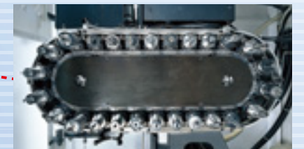
ATC mechanism Tool storage capacity 26(+1)
